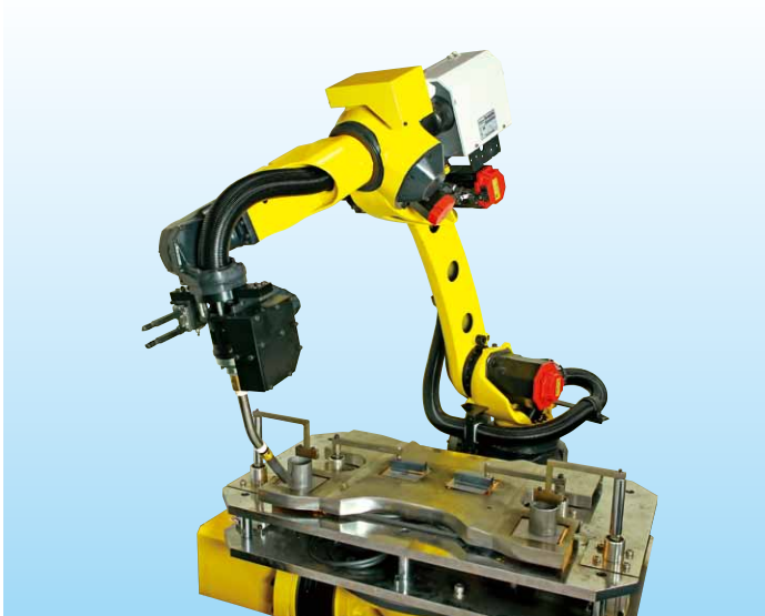
Automotive part welding system
