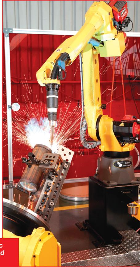
*Robor Pipe Systems' newly acquired robotic welding arm operates at four times the speed of manual welding.*
