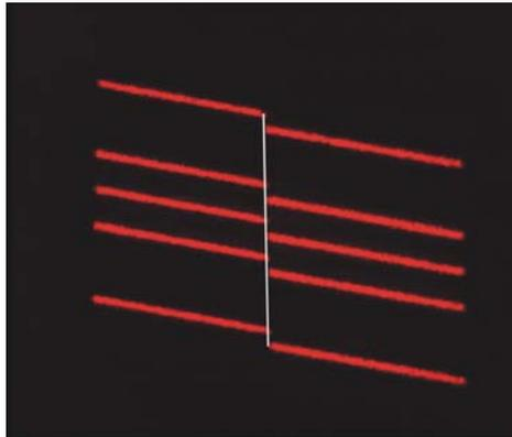
In Figure 3 an angle of approx.  $15^\circ$  is set transversally to the joint direction between the planar workpiece surface and the sensor head.
