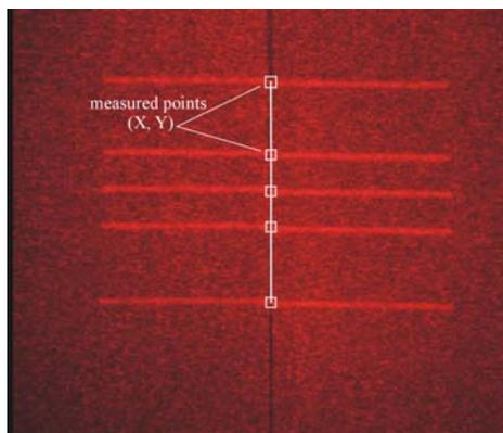
Figure 4 shows the joint recognition for the butt type joint. The tracking of scribed lines or even pencil lines is also possible with these settings.
