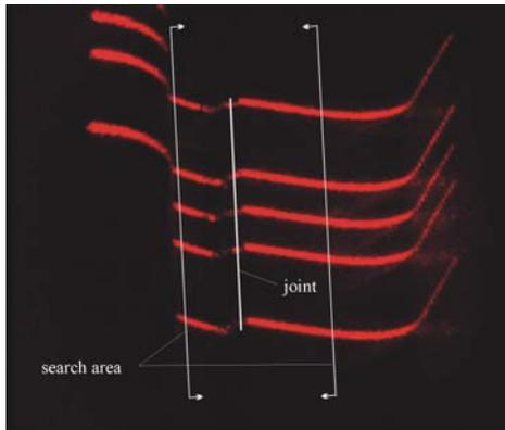
**Figure 1** shows a plate profile and sensor image of a complex joint on two overlapping plates (fillet weld) deep inside a channel in a passenger vehicle roof.
