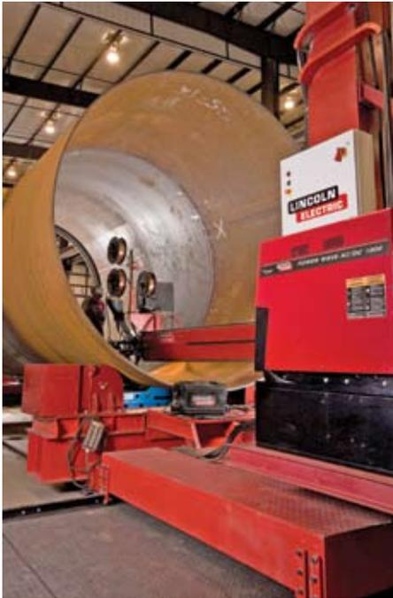
Column and boom installations are ideal for applications involving large parts with long welds.
