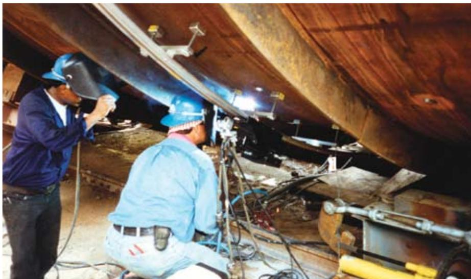
*BUG-O systems – possibly the simplest and the least costly way to automate a welding process. A magnetic BUG-O track is attached along a joint to be welded. All positional welding is possible and weave features are available.*
