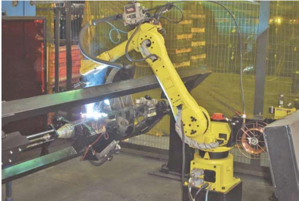
A robotic welding solution by Robotic Innovations with the capacity to handle hundreds of different part sizes and configurations. A Lincoln 355i welding power source is being used to weld truck axles.
